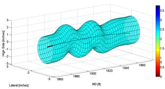
3D representation of transversal displacement. Color temperature is proportional to the maximum diameter of device in inches. At a Measured Depth of 2970.0 ft, the maximum diameter of a device is 2.13 inches, at a device bend of 0.057 degrees / 100 ft. For a device of diameter 3.00 inches, a uniform bend below the allowed maximum was not found.
